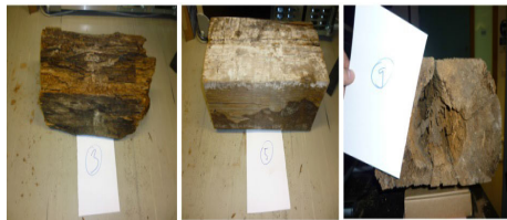
Fig. 3: Examples of wood invaded by decay-fungi and wood-destroying insects.
