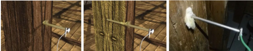
Fig. 4: Temperature diagnostics in a section of a wooden structural element.
